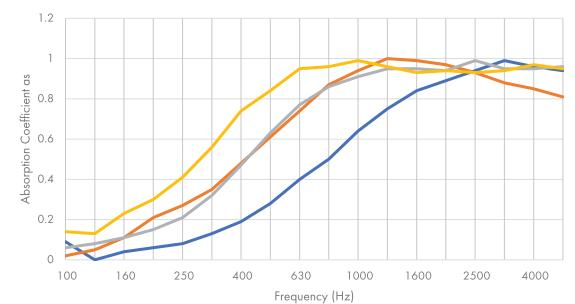
University of Auckland Test Report Number Frequency (Hz) 125 250 500 1000 2000 4000 NRC α<sub>P</sub> 12mm Cube T0712-3 0.05 0.10 0.30 0.65 0.90 0.95 0.45 مp 12mm Cube vith 25mm air gap) T0712-6 0.05 0.30 0.60 0.95 0.95 0.85 0.70 0.95 α<sub>P</sub> 24mm Cube T1316-4 0.90 0.65 <sup>ap</sup> 24mm Cube vith 25mm air go 0.40 0.80
