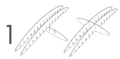
Sort the Lattice 'fins' into pairs, then into size order: largest to smallest. Start by taking one of the largest fins and slotting it into place in the 'rail'.
