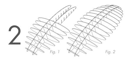
Finish one side by methodically inserting one of each pair into place in order of decreasing size (Fig. 1). Repeat for the other side (Fig. 2).
